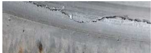
Figure 3 - Failure & Extrication of Shim Plates
