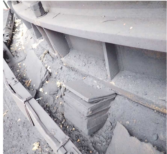
Figure 3 - Failure & Extrication of Shim Plates
